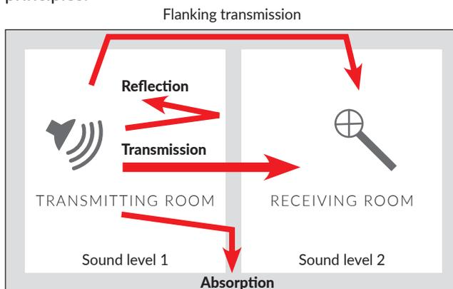
**Mass (weight) of the component:** The heavier the component, the better the sound insulation. To increase the sound insulation, it is necessary for the increase in weight to be significant compared to the original weight. In order to improve a concrete wall with a density of  $200 \text{ kg/m}^2$ , it is necessary to increase the mass by at least  $100 \text{ kg/m}^2$ ; increasing it by  $10 \text{ kg/m}^2$  will have no effect.
